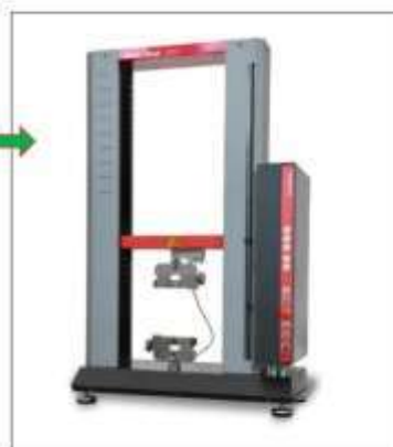
Picture 7: ProLine Z010 after modernization at ZwickRoell's premises
